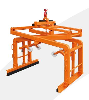
Specifically designed and developed for the UK market to lift palletized brickloads (Note: bricks must be securely bound). Suitable for handling all types of concrete products such as slabs, steel-strapped bricks, blocks kerb stones and paving blocks. palletized bound loads. Lined with hard rubber pads to minimise damage to load.
