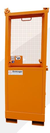
The 1074 1 Man Cage is built primarily with safety in mind, the cage conforms fully to BSEN 14502 and PM28. This cage has solid walled sides to half height and close mesh to the rear to prevent accidental injury but maintain visibility. The cage also benefits from internal overhead harness points.
