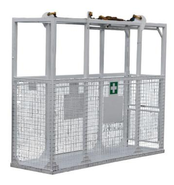
The 1075 stretcher cage is supplied as a crane evacuation cage for use where a casualty needs to be evacuated from height. Suitable for 2 personnel (1 casualty and 1 attendant) and supplied in white with relevant signage. Each unit is supplied complete with four leg chain sling (rated at 10/1 ratio as required by CE regulations) attached to the main lifting points with connectors.
